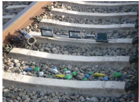
Colour-coded ballast stones for recording behaviour on video as the train passes.
