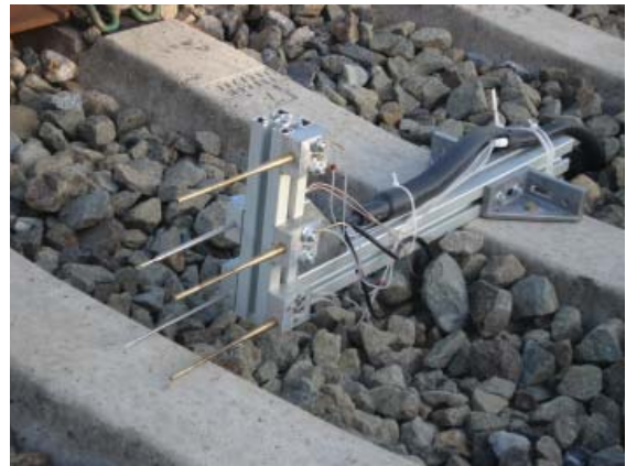
Pitot tubes and hot-wire anemometers installed on the track.
